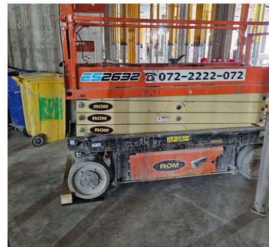
Mobile bump stop to prevent equipment from being able to accidentally hit something.
